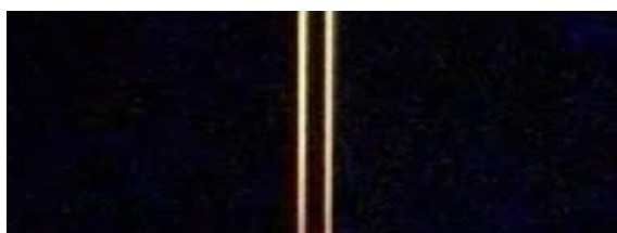
Fig 6.4 (b) Lines Spectrum of Sodium
